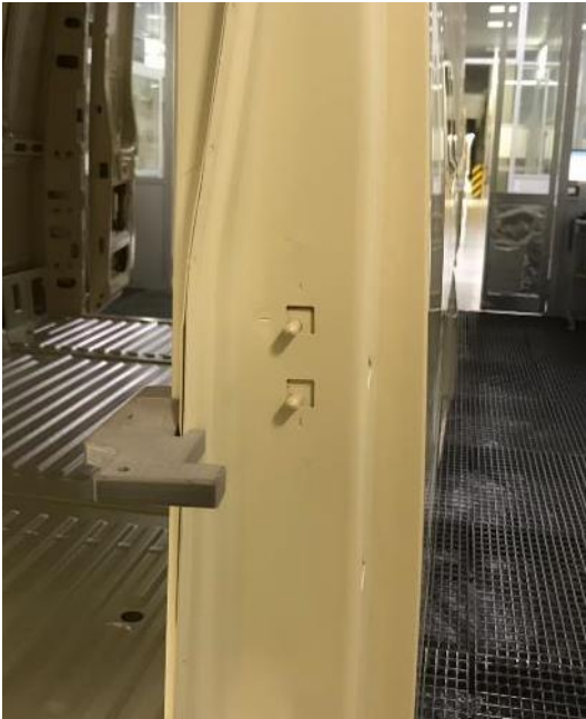
Vehicle door fixture in PEEK
